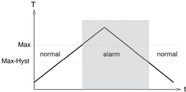
A changeover delay time ( $t_{DS}$ ) can be applied to switching to the alarm state. Equally, one switch-back delay time ( $t_{DR}$ ) of several can be applied to switching back to the normal state.
