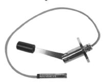
The high temperature model is equipped with only one output (analog output, switching output, or frequency output). Programming is not carried out using a magnetic clip; instead a voltage pulse of 0.5 to 2 seconds is applied to pin 2 of the connector. This model therefore has a different connection mode. The size of the plug gauge (separation of flange surface from fulcrum) of the high temperature model is always 39.5 mm.
